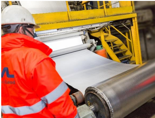
Direct machine cast lead manufacture and coiled
