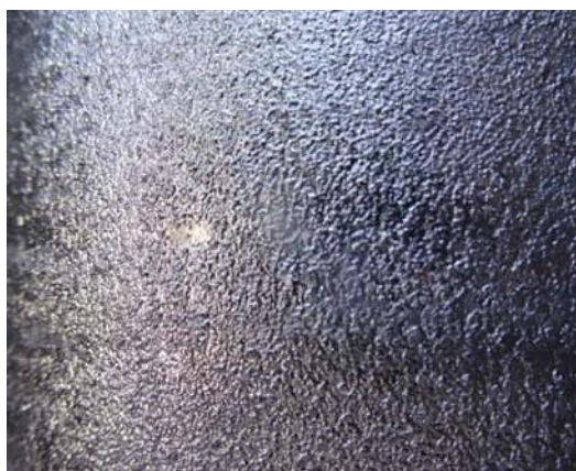
Traditional Cast Lead sand side finish
