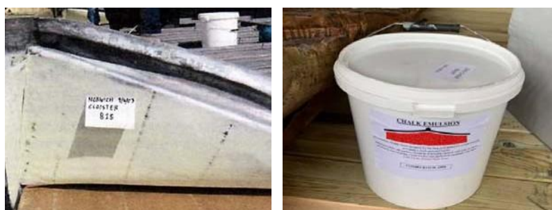
Chalk emulsion coating to underside of lead after 3 years exposure
